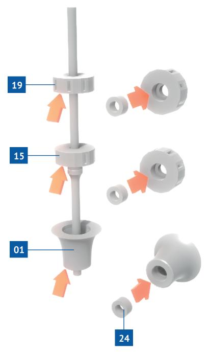
If you do not want to use bearings print part No.24 instead and glue it to the shaft to hold it in place.
