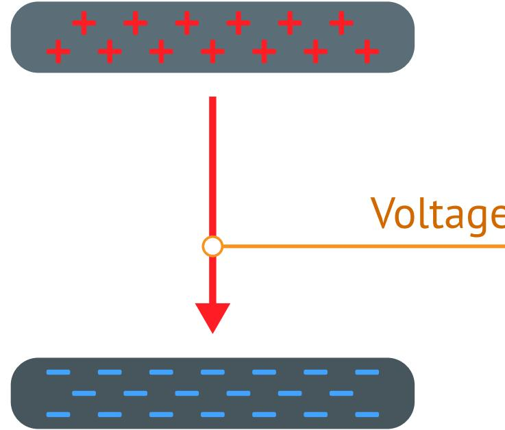
A high voltage is applied across a tube filled with gaseous deuterium.
